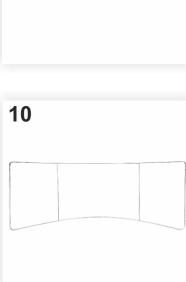
7-8. Mount the corner elements at the ends of the two curved bars thus obtained.
